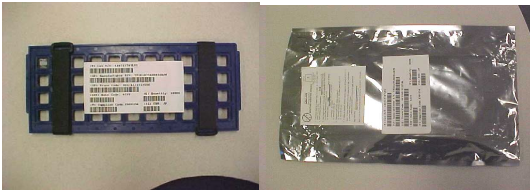
Figure D-5: Example of preferred tray labeling. Photo on the left shows label on top cover of tray. Photo on the right shows a redundant label on the ESD / Moisture Barrier Bag which typically contains trays of components.
