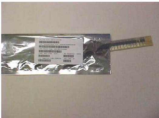
Figure D-4: Example of alternate labeling method when individual tubes cannot be labeled – Each tube is placed in a protective bag labeled as per this specification.
